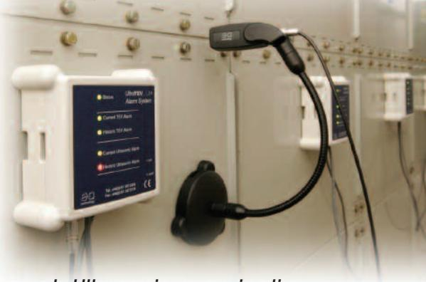
*Transient Earth Voltage testing is complimented with a thorough Ultrasonic examination. We regularly work with our customers to identify the component under stress and often provide follow-up testing to ensure it has been effectively dealt with.*
